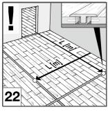
**Installation:** It is recommended that you lay out the panels in the direction of the length and the source of light [11].
