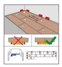
Proceed in the same way when inserting the next rows. Make sure that the boards are absolutely flush with each other. Make sure that the offset of the head joints from row to row is at least 30 cm.
