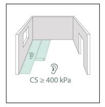
The use of a suitable impact sound insulation for vinyl floors is necessary. Please use an impact sound insulation with a pressure load of min. 400 kPa.
