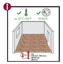
Please note that typical living room temperatures must prevail throughout the year (VOB, Part C, DIN 18365, DIN EN1264, DIN 4725). The room air temperature should be approx. 20°C, the relative humidity should be between 35-60%.
