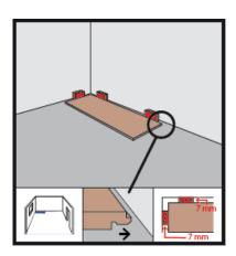
The first row is laid so that the spring of the head and long side faces the wall. Fix the first row with spacers (min. 7 mm) to the wall.
