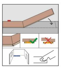
Click the front side of the panels into the previous panel at a slight angle. Make sure that the panels are absolutely flush with each other.
