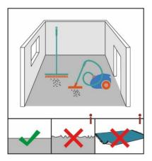
The substrate must be crack-free, clean, tension/compression resistant and completely dry (VOB, Part C, DIN 18365). Before laying, remove all old floor coverings from the subfloor as far as they may affect the evenness of the subfloor. The evenness of the substrate should not deviate by more than +/- 3mm on 1m (DIN 18202).
