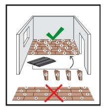
Before laying, check each individual board for colour and structure. It is advisable to mix several packages in order to obtain a uniform laying / sorting pattern.
