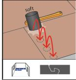
The first panel of the second row is attached to the first row by angling it along the long side. To do this, place the longitudinal tongue at an angle from above into the longitudinal groove of the first panel of the first row. Then lower the panel until it lies flat.
