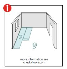
The use of a suitable impact sound insulation for vinyl floors is necessary. Please use an impact sound insulation with a pressure load of min. 200 kPa.
