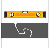
Then carefully knock into place using an acrylic hammer. This makes installation easier and ensures that the front-end connection is locked completely and accurately. Make sure that the panels are absolutely flush with each other.
