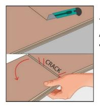
The custom-made panels are easily shortened with an angle and a carpet knife. Alternatively, you can also use a laminate cutter or a jigsaw. The panel is then "broken over the edge".
