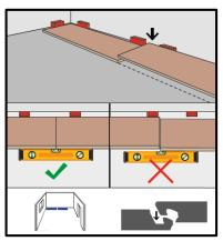
Click the second panel into the previous panel on the front side. This is done from above by gently pressing it in by hand until the click connection latches into place.
